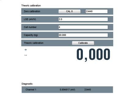
Inside this menu you can see the mV of the Load cell and also the internal Counts. In case of an error of the scale you can check here if the Load cell is working properly.
