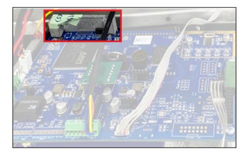
Now lift the Jumper of the Calibration-switch and place it again.
